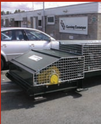
Tail Unit - with Rulmeca non drive drum, and feed boot
