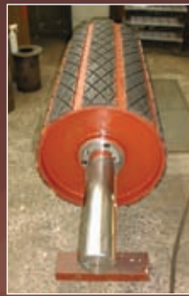
HEAD DRUM WITH SLIDE LAGGING AND TAPER LOCKS
