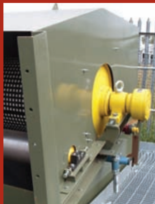
SuperDrive drum in retro-fit with Ceradrive lagging
