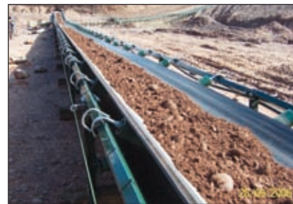
Complete Canning Field Conveyor Bays (900mm belt - steel safety handles - in 2.6m long bays).
