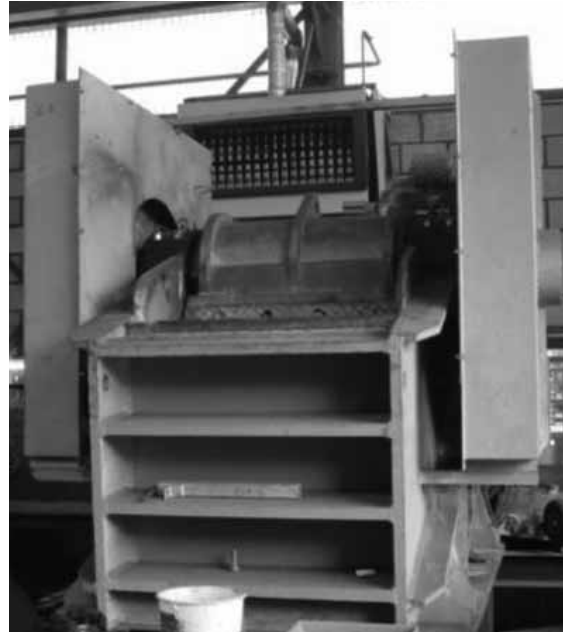
Granulator Jaw Crusher, Aubema, like new inlet = 1000 x 350 mm incl. Hydraulic adjustment, grease lubrication with motor Price £42,000 Ex site
