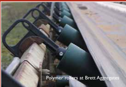
Polymer rollers installed Goddards Quarry
