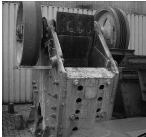
JAW CRUSHER, WITH MOTOR INLET = 800 x 630 mm Price £26,000 Ex site
