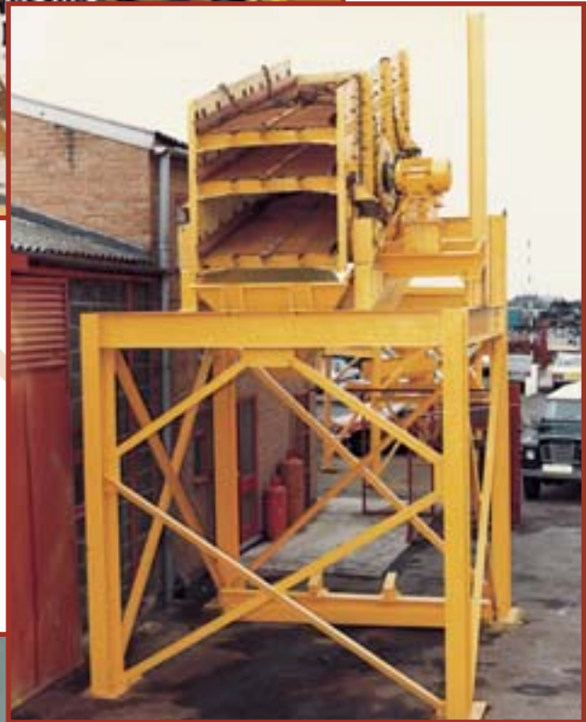
▶ 3-deck screen and supporting structure
