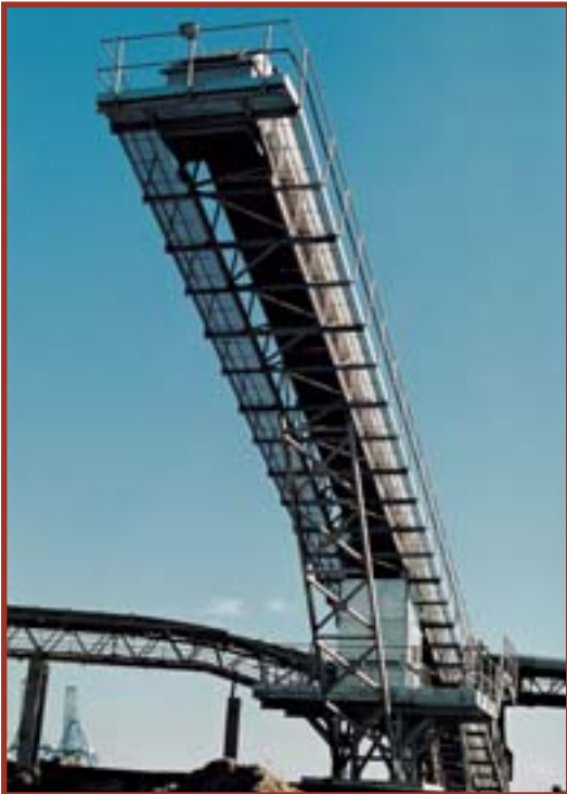
5000 tonne galvanised stockpile conveyor handling 1800 tph of sea dredged aggregates supplied to Brett Aggregates Ltd.
