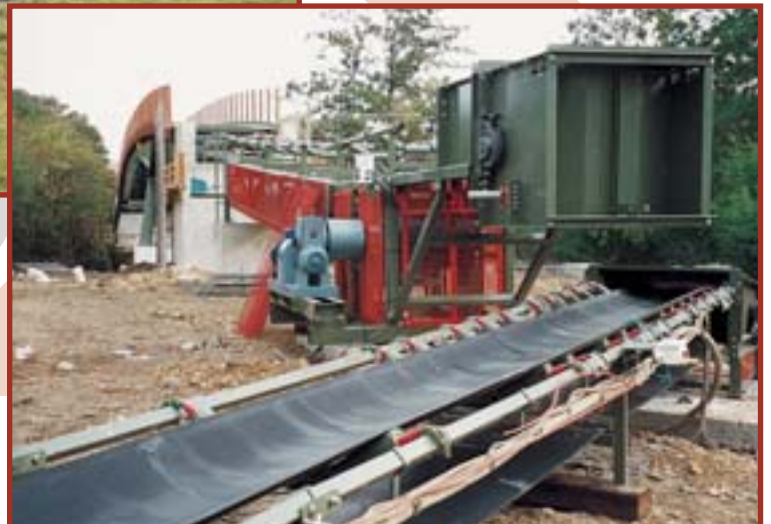
Field Conveyor crossing new bridge over River Thames, supplied to Summerleaze Ltd.
