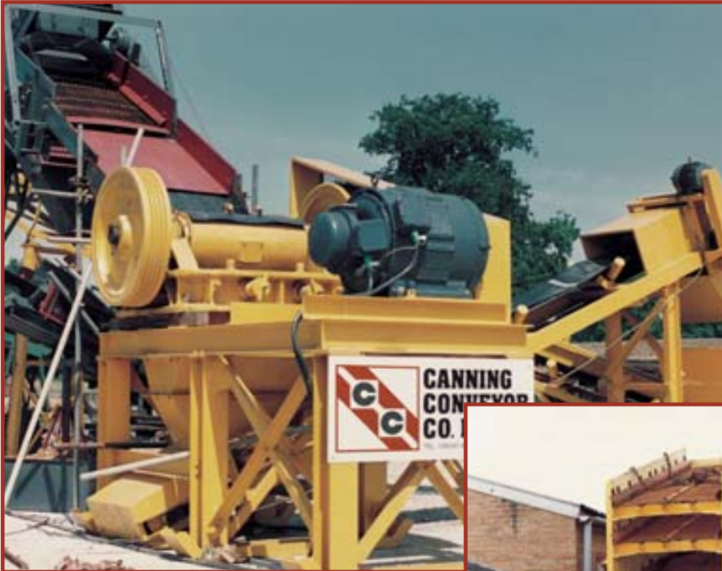
▲ Static Crusher and Conveyor for M25 improvement project
