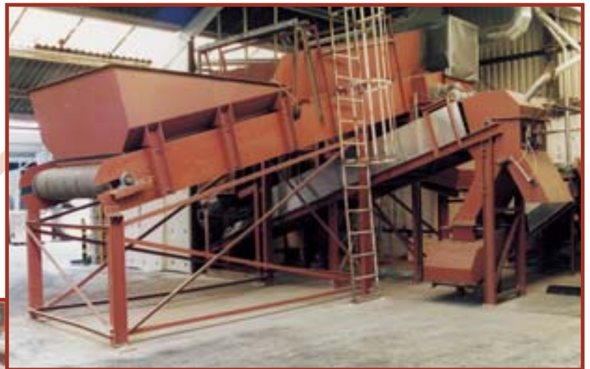
Fully integrated Cable Granulation Plant supplied to Thomas Bolton Process Metals Ltd.
