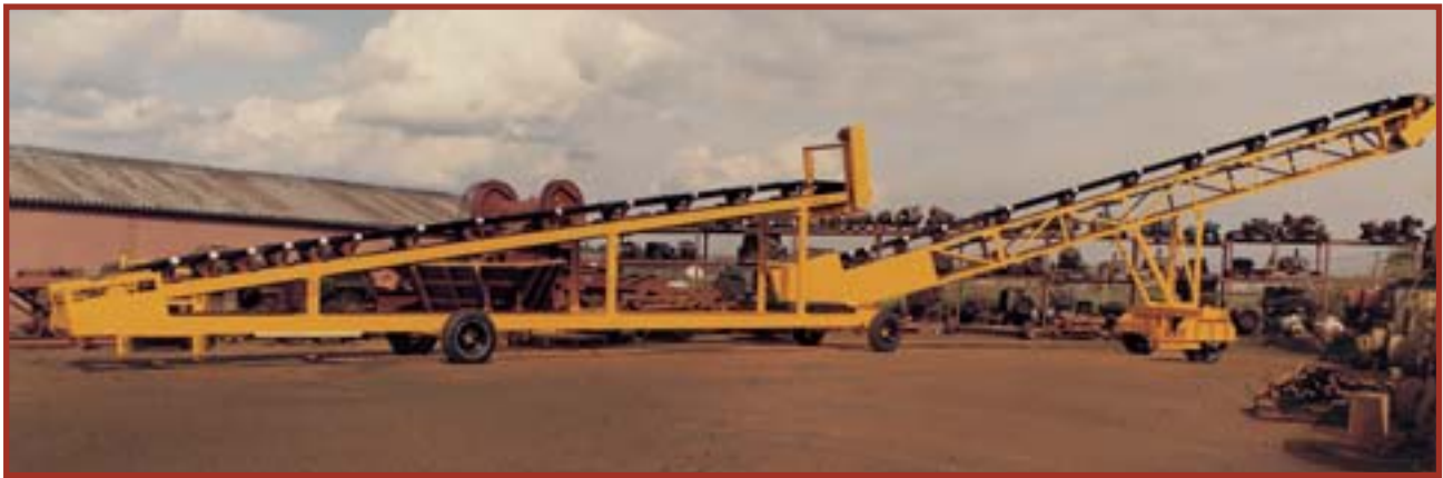
▼ Mobile linking conveyor as part of a snake system, supplied for operation in Iceland
