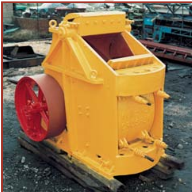
▲ Fully refurbished 36 x 24 KueKen Crusher
