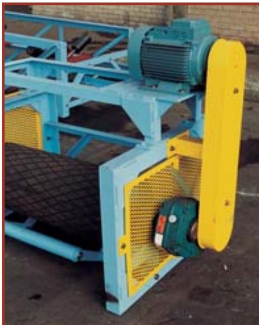
◀ Full drive assembly incorporating drum, bearings, drive frame with motor, vee belt, shaft mounted gearbox and guards
