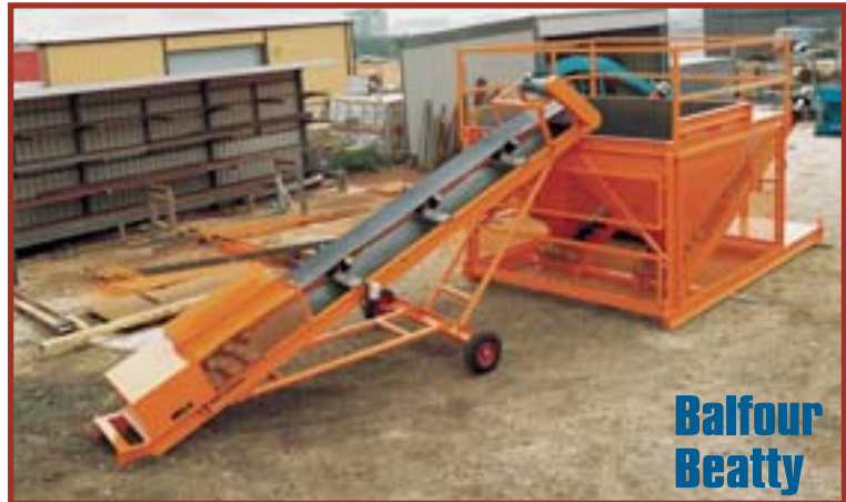
▲ Mobile Feed Conveyor and skid mounted hopper/conveyor unit handling shotcrete, supplied to Balfour Beatty.
